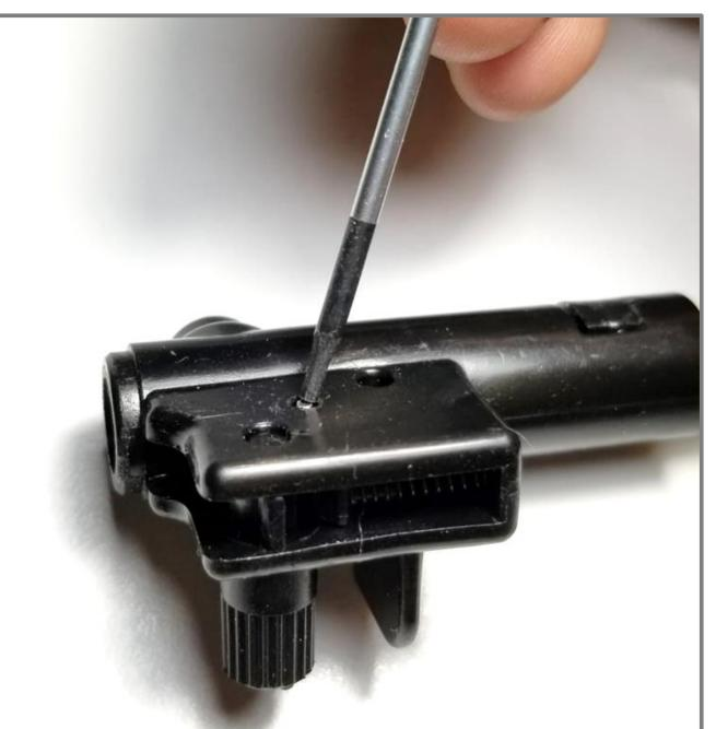
Remove the hop up arms pin. You can use a thin screw driver to punch it through.
