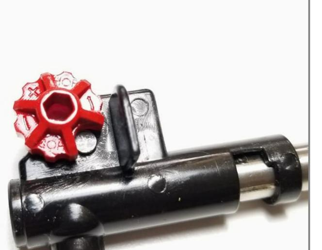
Apply pressure to ensure the whole pin is fully inserted into the hole.
