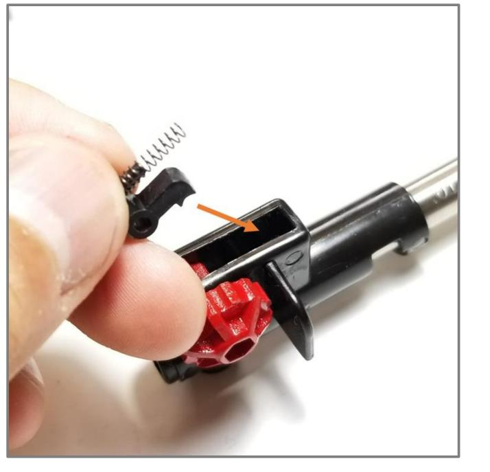
Insert the hop-up arm directly in to the hop-up unit slot downwards. Ensure the spring is against the wall of the unit.
