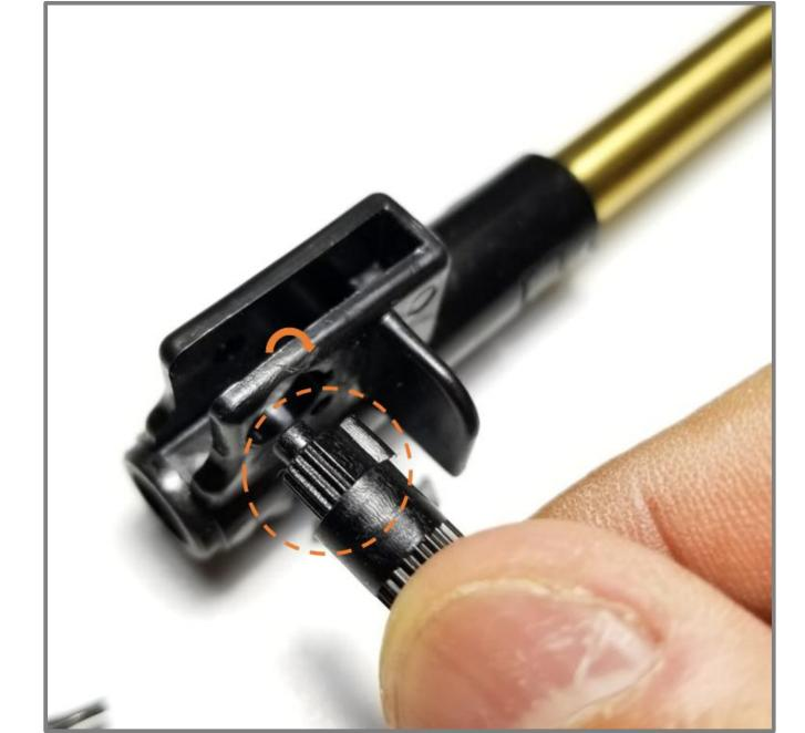
Twist the adjustment knob 90 degrees to the right until it reaches the slot enabling it to be pulled out.
