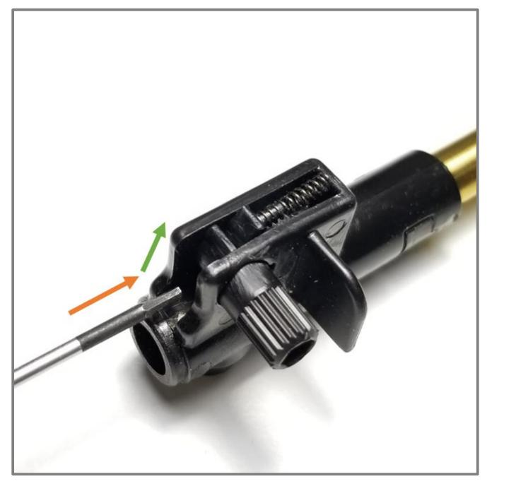
Next, removing the hop-up arm. Use the screw driver to insert into the hop-up unit underneath the adjustment knob. Tilt your screwdriver and push up. The hop-up arm will then pop out easily.
