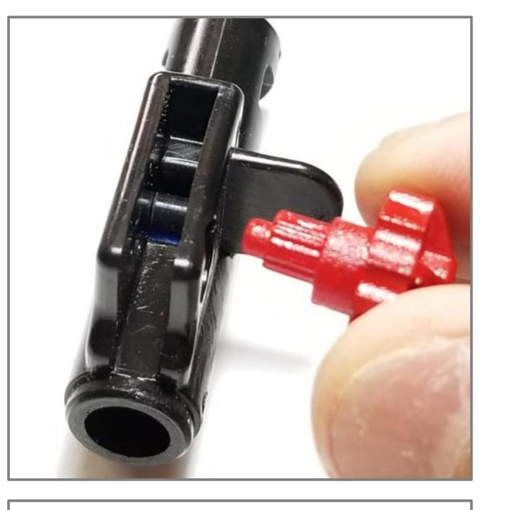
Insert the upgraded Airtech Adjustment knob into the hopup unit.
